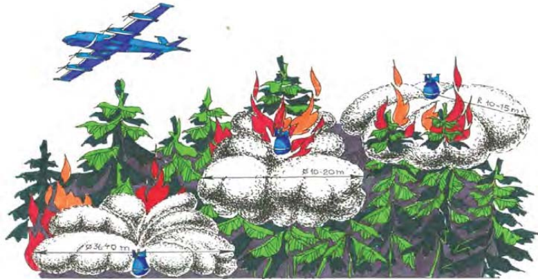
Pict. 5. First stage of PFFFT is stop and localization of upper fire's front by bombing with numerous "TSA-500" precisely bombing from safety height 2-4km.
