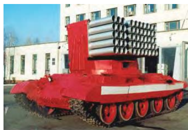
Pict. 10. Multibarrels unit on the tank-chassis for protection of military, industry, government, nuclear power stations, villages, cottages, suburbs from forest-fires.
