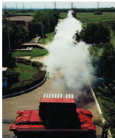
Pict.9. At first all over World – instant for 1sec: extinguishing local fires at area of 15m 2 with 2kg dust and 1,1m 2 scorched wood with single liter of clean water.
