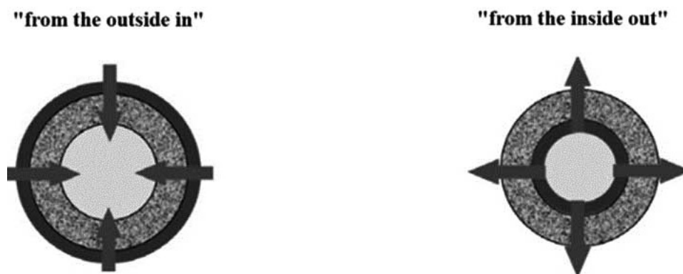
Fig. 3. Type of filtration through an ultrafiltration membrane
