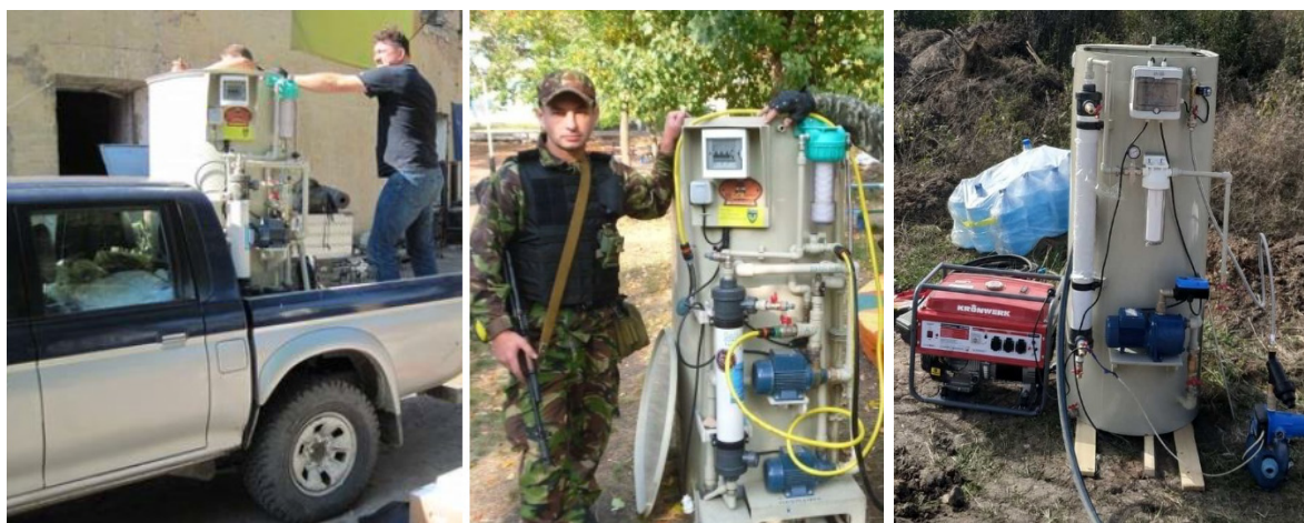
Fig. 1, 2, 3. Autonomous mobile pilot unit for combined filtration and electrochemical water treatment to drinking water standards
